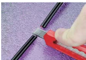
Figure 1. Slice the POF cable.
