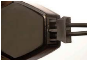
Figure 3. Insert POF into OptoLock.
