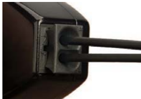
Figure 4. Press OptoLock to hold POF into place.
